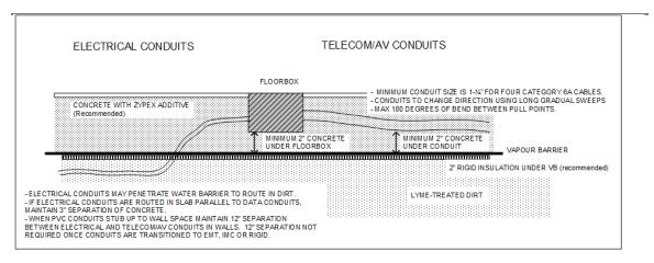
All floorboxes in a slab over grade shall be designed and built according to this drawing.
